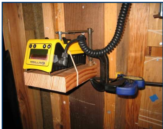
Testing the microwave device and its ability to detect drywood termites
