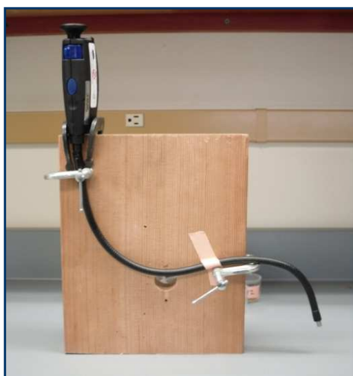
Boroscope set-up for the bench top exercise
