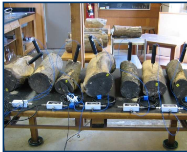
A computerized Acoustic Emission Device (AED) monitoring drywood termite feeding patterns.
