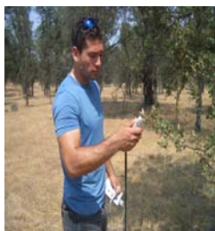
This picture illustrates the porometer that reads the Stomatal conductance of leaves- being used by me at the Tonzi Field.
