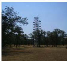
These two pictures illustrate the seasonal changes in the Tonzi Field and the tower where it measures the Eddy Covariance and \text{CO}_2 content of the canopy.
