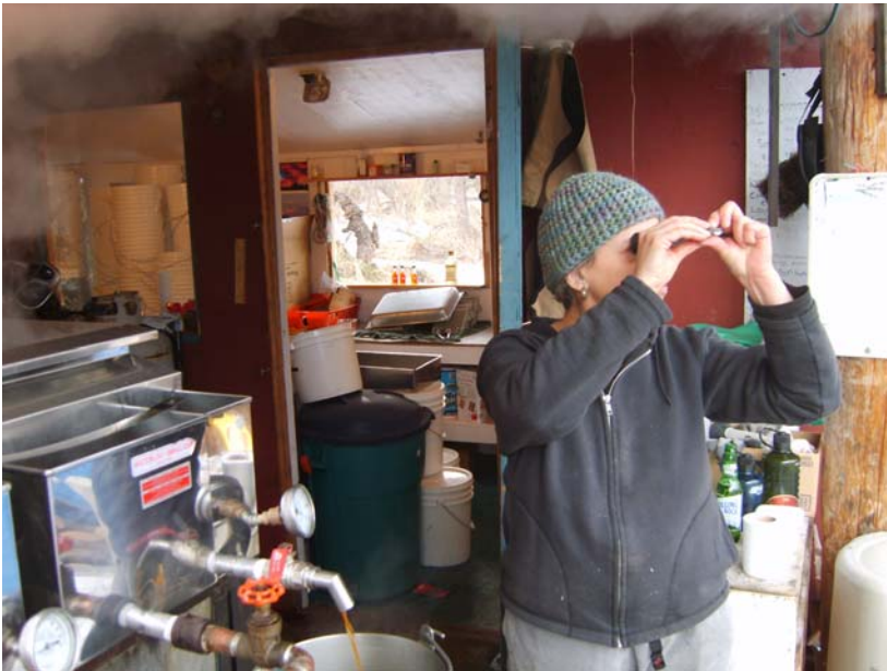
Dulce Ben-East of Kahiltna Birchworks testing the sugar content of birch syrup being drawn of the wood-fired evaporator.
